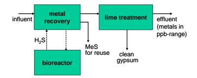
Figure 5. Biological metal recovery applying the S-cycle in anaerobic technology.
