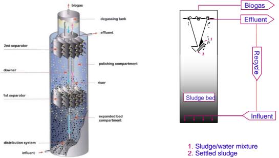
Figure 2. Paques IC reactor (left) and Biothane EGSB reactor (right), inoculated with granular sludge. Applicable loading rates: 15-45 kg COD/m<sup>3</sup>.day.
