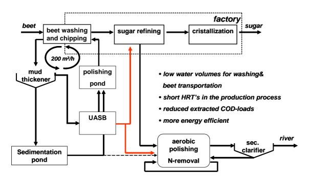
Figure 4. Implementing anaerobic high-rate technology for optimising internal water loops in sugar beet processing industries.
