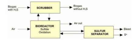
Figure 4. Biogas desulphurization unit combining an alkaline scrubber with a partial oxidation of HS<sup>-</sup> and alkalinity recovery.
