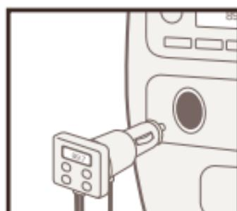
The transmitter's antenna is in the cable that connects to your Zune. To improve reception, try moving Zune farther from the transmitter.
