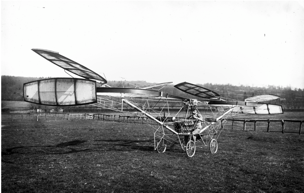
Figure 20: The completed Cornu helicopter in 1907, with pilot on board, apparently ready to fly.
