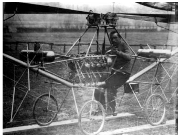
Figure 17: A close up view of the Antoinette 8-cylinder engine, and the pilot's station with the flight control levers.
