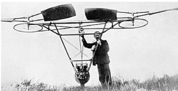
Figure 8: Charles Renard built this machine in 1904, which had two rotors of 2.5 m diameter. It did not fly successfully.
