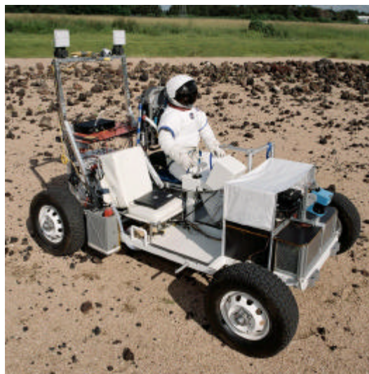
4-10: Fuel Cell-Powered Rover Development for Future Human Space Exploration
