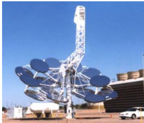
4-4: Concentrating Solar Collector
