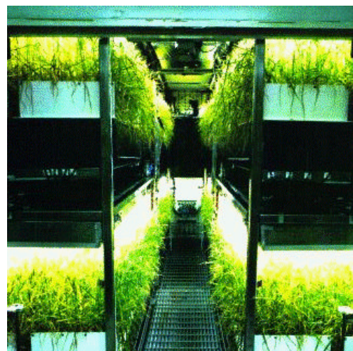
2-1: Closed Chamber Testing at JSC Using Machines and Plants to Recycle Water and Air
