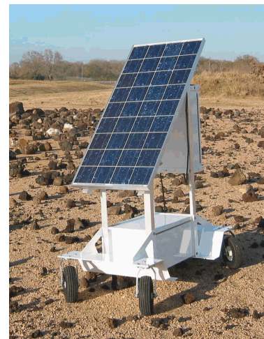
6-3: Solar-Powered Recharge Station at JSC's Mars Terrain
