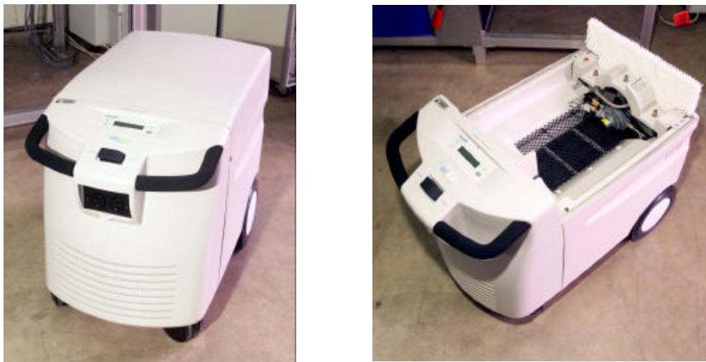
6-5: Commercial Fuel Cell UPS Installed to Back Up Power for a Test Computer at JSC
