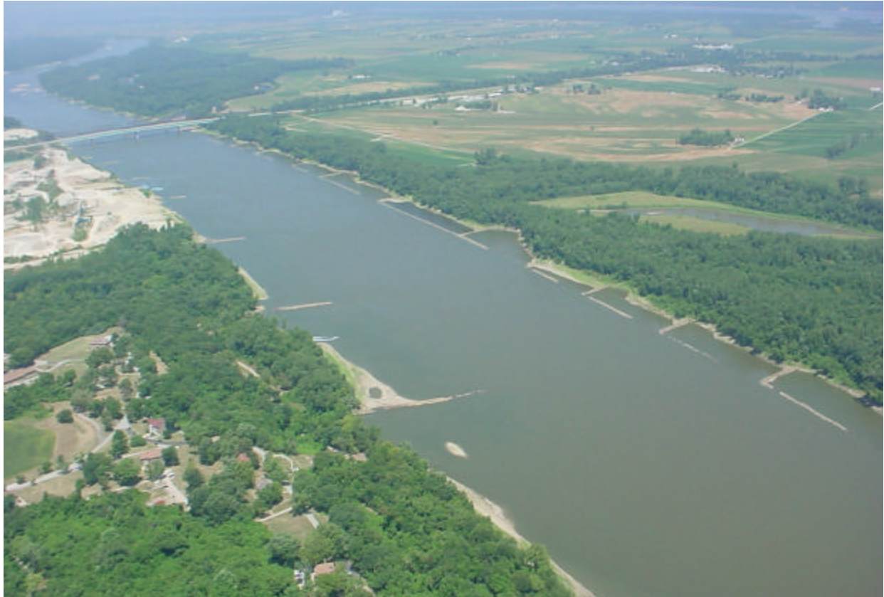
Figure 2: Photograph of the Missouri River north of St. Louis, looking northwest from a position near Mile 6.5 at an altitude of 1500 feet, during the low flow conditions of July 31, 2002. Lewis Bridge on US 67 is in the middle background (Mile 8.2). Note the prominent wing dams located every 600 to 1200 feet along both sides of the river; the tree line on the north side marks the approximate position of a levee. The site of Fort Bellefontaine is located in the left foreground and is proximal to the first and last campsites of the Lewis and Clark expedition (May 14, 1804 and Sept. 22, 1806). Photo by author.
