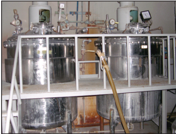
Figure 4. Two 1,000-liter, stirred, jacketed vessels suitable for use as fermentors for the growth of bacterial BW agents.
