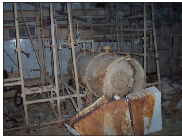
Figure 15. Reactor made from recycled two-ton bulk mustard storage cylinder.
