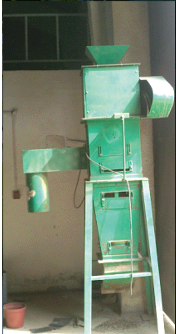
Figure 5. Thresher used to mash castor beans found at TABRC.
