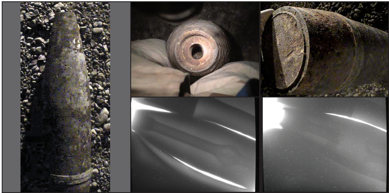
Figure 5. Examples of the 10 155mm chemical rounds and x-rays of ruptured burster tubes.
