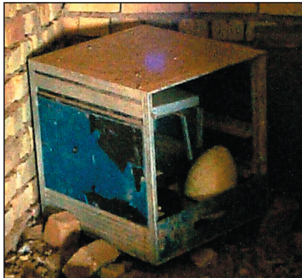
Figure 21. A Skinner Box, a device used to test small rodents who are under the effects of drugs or chemicals, was recovered at one of the sites.
