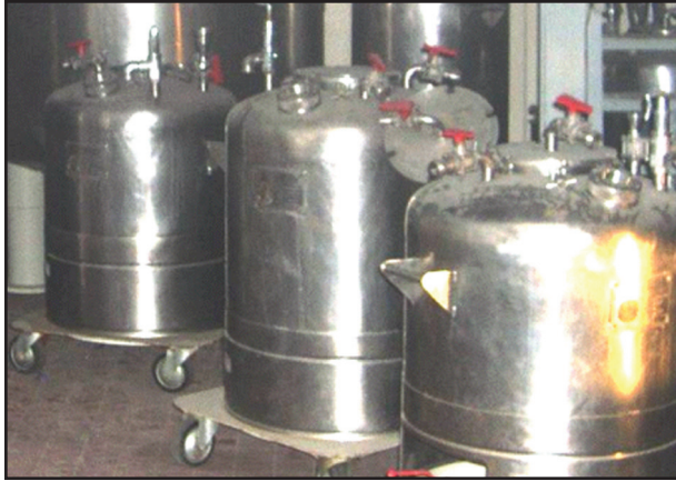
Figure 13. 1m 3 Stainless steel mobile tanks.
