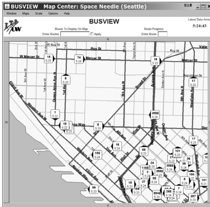
Figure 2-8: Wireless technology tracks city buses in Seattle and reports locations on a website.
