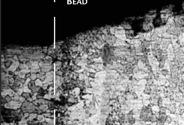
Recrystallization of 7005 aluminum after welding leaves enlarged grain susceptible to cracking.
