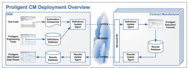
You can deploy Proligent on a few test and assembly stations, on a complete production line, or at contract manufacturer's site. Usage can be expanded as needs evolve.
