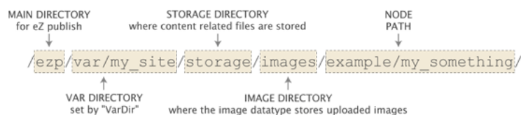
Figure 5.21: Example of image path on the filesystem.
