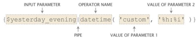
Figure 3.8: Typical components of a template operator call.
