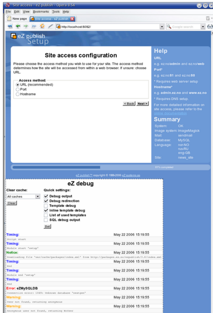
Figure 1.27: The debug output appears at the bottom of the page
