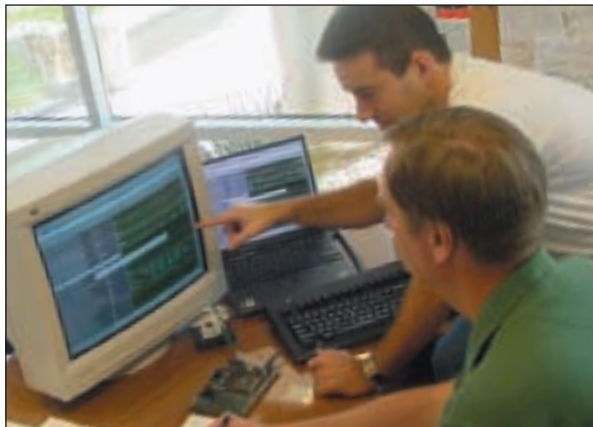
Insight Engineers Jay Seashore (seated) and Donny Saveski examine a Modelsim waveform simulation of a TxPhy.
