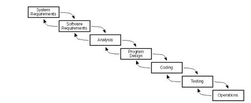
Exhibit 2—View by W. Royce (1988b, Figs 2 and 3) of the implementation steps to develop a large computer program for delivery to a customer, with iterative interaction
