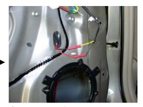
Connect wires (make sure to confirm +/- polarity) – my connections as shown were to a crossover. The car's black is + and yellow is -, connected to my crossover's red + and black – (always interesting <u>not</u> connecting black to black...)
