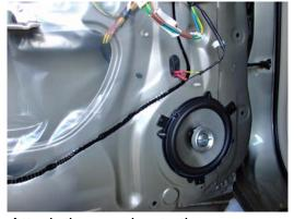
Attach the speaker to the mounting bracket using the four screws as provided. Be careful – this is the closest you will come to the delicate neoprene of the speaker cone with a sharp object!
