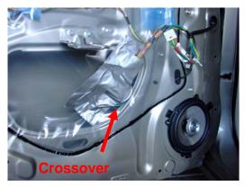
Cut a small slit to bring the crossover back thru to the front of the plastic. Tape the crossover to the plastic using duct tape. Use the same duct tape to re-seal the door.
