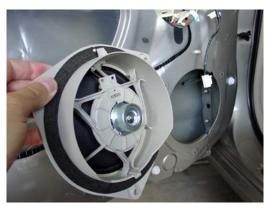
Remove the speaker – amazing how small the magnet is on the back is, and how light the entire speakers is – no wonder it sounded like that!
