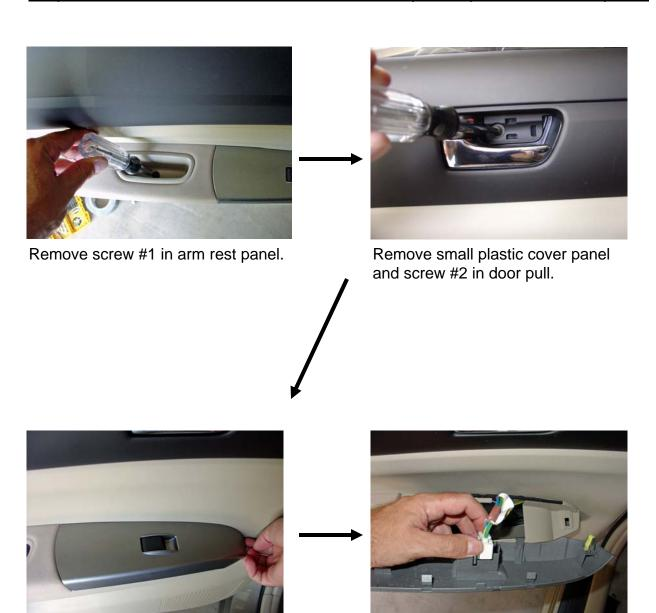
Remove arm rest panel – up gently on forward edge – it snaps out very easily,
