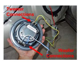
Connect crossover wiring to the new speaker – this one has two connections for the tweeter (yellow and green) and two for the woofer (white and blue). Make sure to confirm +/- polarity.
