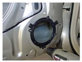
Attach the new plastic speaker mounting bracket provided (pictured above) – use two of the existing holes you just drilled the rivets out of, and drill one new one. Attach with three new screws and clips in the back (as provided).
