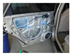
Photo of door with panel removed. I had a few *stubborn* white clips stay in the door – remove them from the door by pushing from the inside out – and re-attach them to the door panel.
