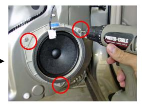
Using a 1/8" bit, drill out the rivets – this requires a little elbow grease – don't be gentle. Retrieve any loose parts that fall into the door (so they don't rattle around later as you drive around).
