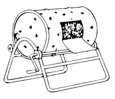
Figure 1. Rotating barrel composter.
