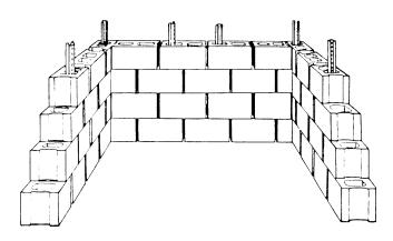
Figure 9. Cement block holding unit.
