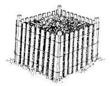
Figure 8. Snow-fence holding unit.
