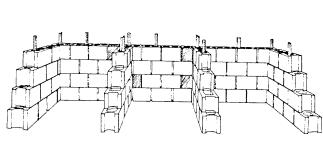
Figure 5. Cement block three-bin composting unit.
