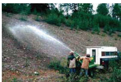
Figure 4: A small "research class" hydroseeder being used by Plant Materials Center staff in a Southcentral gravel pit plot.
