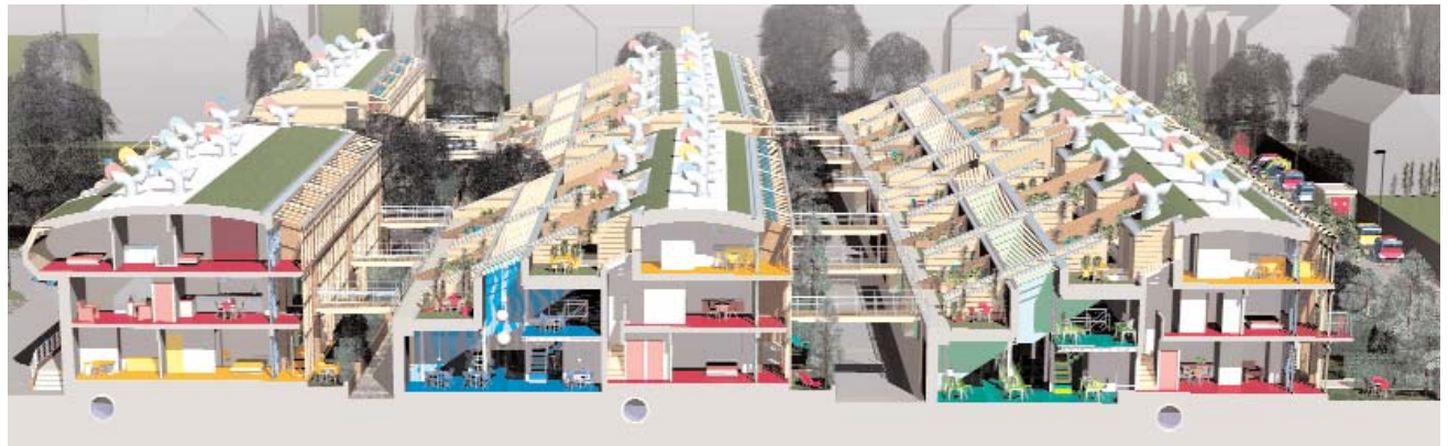
Below: The section through the BedZED scheme underpins the whole ZED approach - Solar orientation with homes facing south & workspaces north with skygardens on their roofs. All upper roofs are green sedum and there is a full range of unit types and tenures
