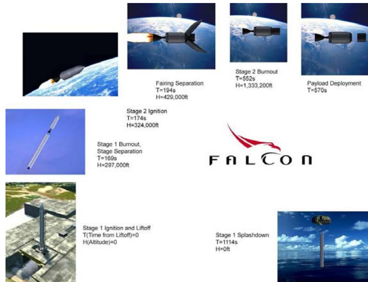
FIGURE 5-4: FALCON 1 SAMPLE FLIGHT PROFILE, DIRECT INSERTION MISSION
