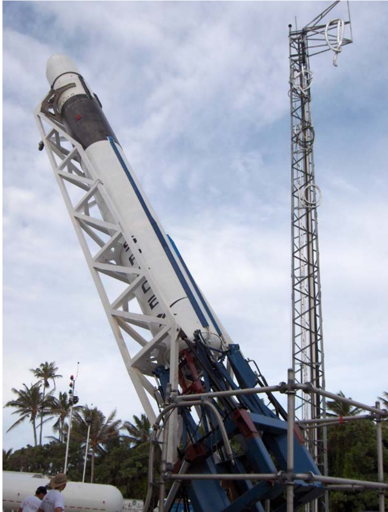
FIGURE 5-2: ERECTION OPERATION ON OMELEK ISLAND WITH LAUNCH VEHICLE AND TRANSPORTER ERECTOR
