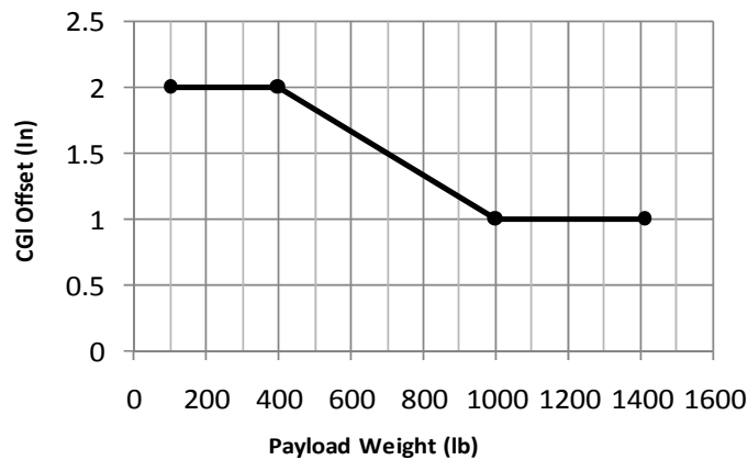
FIGURE 3-1: ALLOWABLE CG OFFSET FROM CENTERLINE
