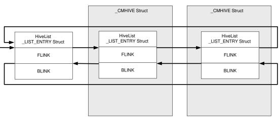
The CmpHiveListHead variable is simply a pointer to the List Head \_LIST\_ENTRY structure. In a sense the job of the List Head is to point to itself when the list is empty.
