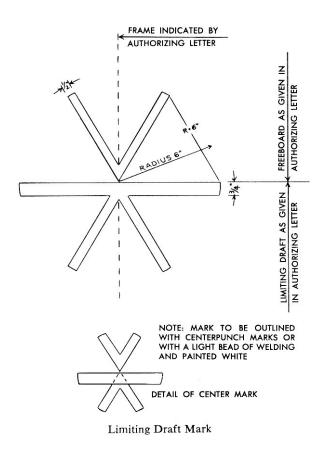
Draft figures on metal hulls will be made by running a bead of weld around the outline of draft figures projected on the hull. The figures shall be located so that the bottom of the figure is tangent with the draft it represents measured from the bottom of the keel line extended. Draft figures shall conform to Coast Guard Plan No. FL-2 804-15.
