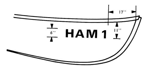
Identification markings for boats 20 feet and over and assigned to named vessels.
