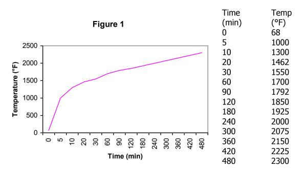
The furnace interior temperature during a test is controlled such that the area under the time temperature curve is within 10% of the corresponding area under the standard time temperature curve for 1 hour or less tests, 7.5% for those less than 2 hours and 5% for those tests of 2 hours or more duration.
