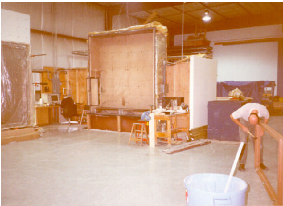
Figure 1 – Smoke leakage testing apparatus (ITS Middleton, WI, USA)
