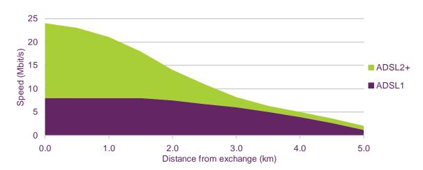
Figure 4.4 Theoretical maximum DSL speeds by length of line from exchange to premises
