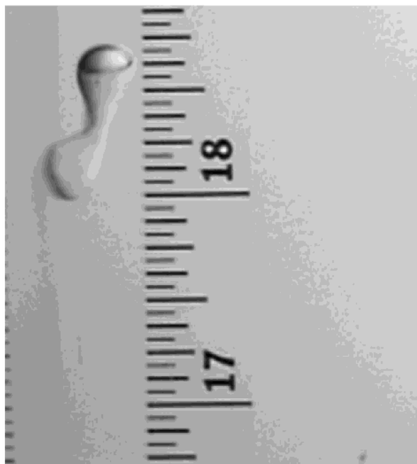
FIGURE 5. CO 2 droplet evolution in crossing the liquid–gas-phase boundary, while still within the hydrate stability zone.
