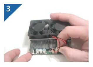
3. Attach the cables to the connectors on the processor upgrade
