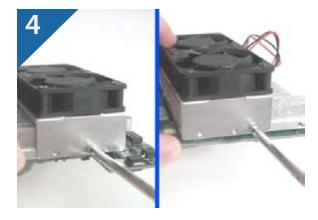
4. Attach the fan to the heatsink as shown in the picture, using the screws provided. Make certain you do not cover the hole used to attach the upgrade to the logic board.
