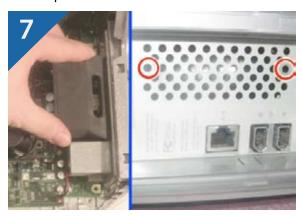
7. Replace the black shrouded fan back into position and replace the screws on the back of the chassis. You're done!
