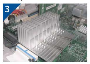
3. Remove the heatsink clip and lift the heatsink off the processor module.
