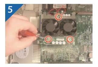
5. Using the original processor screws, secure the new processor to the logic board as shown in the picture.
