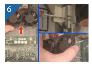
6. Slide the fan assembly over the heatsink as shown in the picture. This will cover the third screw hole. Attach the screws to the each side to secure the fan to the heatsink.
