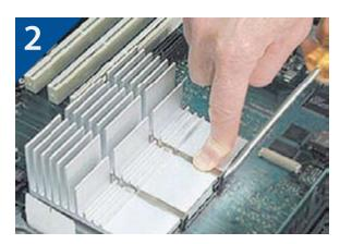
2. Press down on the top of the heatsink clip, use a small flatblade screwdriver to lift up and out on the front tab of the clip to release it.
