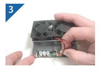
3. Attach the cables to the connectors on the processor upgrade .
