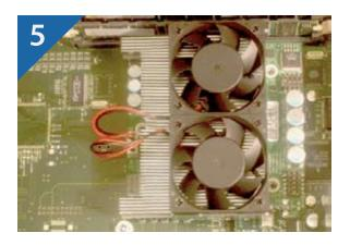
5. Locate the connector on the logic board where the original processor was installed. Line up the new processor as shown in the picture. Once lined up, firmly press down on the screw holes. You will hear the processor snap into position. Using the original processor screws, secure the new processor to the logic board as shown in the picture.
