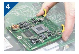
4. To disconnect the processor from the main logic board, hold it by the edges nearest the two opposing screw holes (on either side of the connector), gently rock the processor right to left, and lift straight up. If your computer's configuration has RAM installed that makes it difficult to hold the processor correctly, remove one row of RAM to give you better access.
