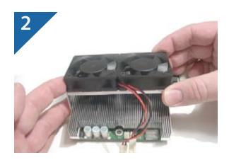
2. Place the fan over the heatsink as shown in the picture, with the cables facing the single screw hole.
