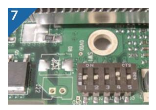
7. Locate the DIP switch in the lower lefthand corner. Set the switches according to the chart.
