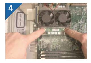
4. Locate the connector on the logic board where the original processor was installed. Line up the new processor as shown in the picture. Once lined up, firmly press down on the screw holes. You will hear the processor snap into position.
