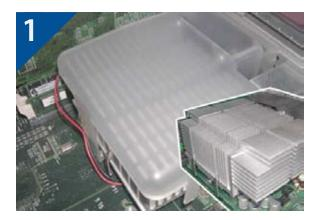
Locate the heatsink. [On Digital Audio unplug the fan connector, release the plastic tabs from the processor card, then remove housing. On Quicksilver: remove screws on rubber fan housing through grill at the back of the computer. Lift straight up to remove.] You will be replacing this fan assembly after installing the upgrade.
