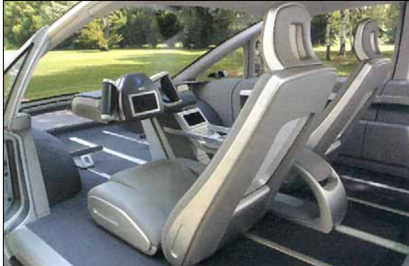
Fig 20 – Interior of Drive-by-Wire Vehicle showing Increased Driver Space
