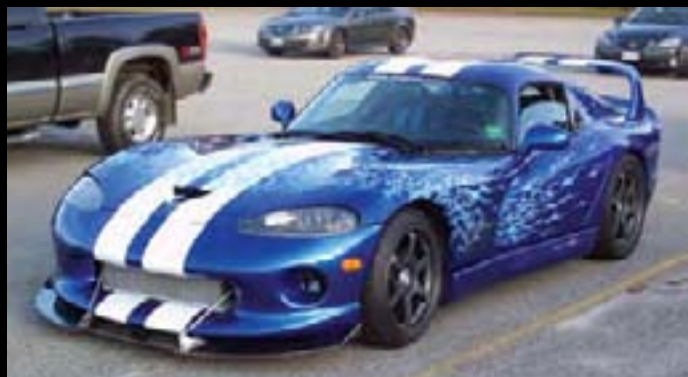
LOT #644 - 1996 DODGE VIPER GTS TWIN-TURBO COUPE A 1300hp Twin-Turbo Viper with a top-mount Turbo design, huge front mount inter-cooler and all the supporting mods including Aeromotive fuel system, spec twin disc clutch, roll cage, upgraded transmission and Unitrax rear end with hardened gears.
