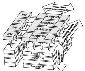
Spatial index structure traversal on such a SPU would not be very efficient since this requires a significant number of scalar floating point operations, while an SPU is optimized for vector operations. For this reason a specialized Traversal Processing Unit is also present to do this task. This Traversal Unit is called with a special instruction on the SPU, which then runs another thread while waiting for the results.
