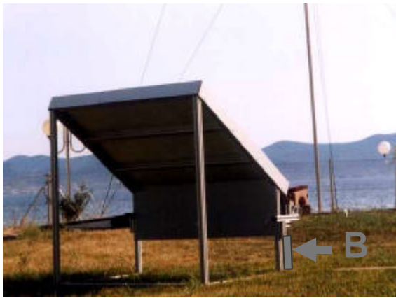
Figure 2. The dew condenser at the Zadar station (Croatia). B is the bottle for dew volume measurement.
