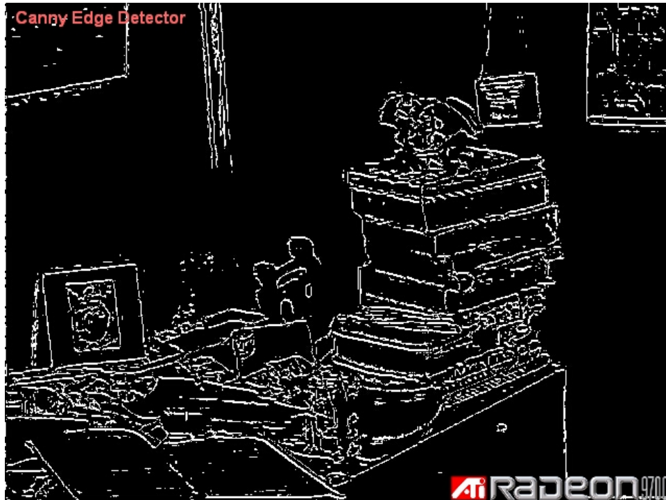
Figure 4 - One-Pixel-Wide Edges from Canny Filter
