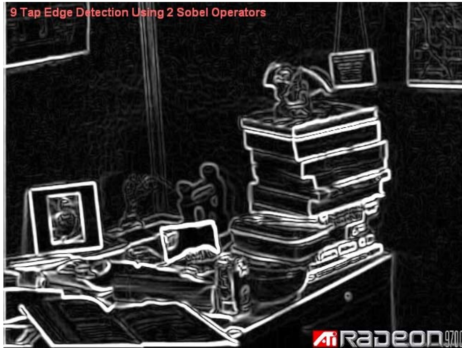
Figure 5 - Gradient Magnitudes from Sobel Filter (see [Mitchell02] )
