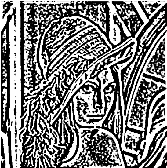
Figure 14 - 17×17 Laplacian of Gaussian Operation
