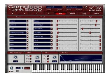
The Mod page allows you to map a range of control sources to various modulation targets (i.e. Voice Program parameters).
