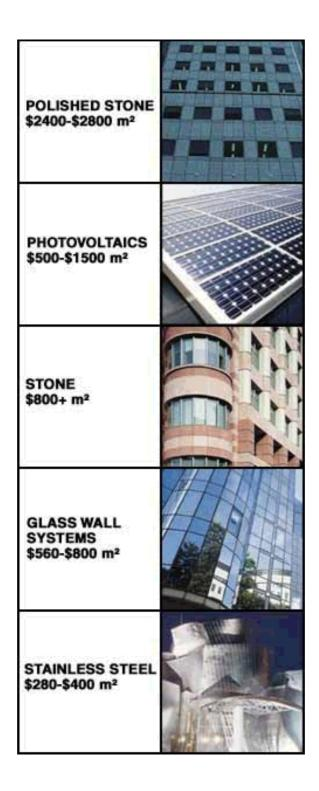
Figure 3.1: Reference costs of façade cladding materials (source..)
