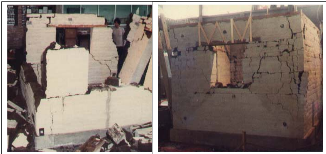
FIGURE 18 – Seismic Performance of an Unreinforced Adobe Building (Left) and a Strengthened Adobe Building with Internal Cane Reinforcement and Ring Beam (Right) (Blondet et al, 2002)
