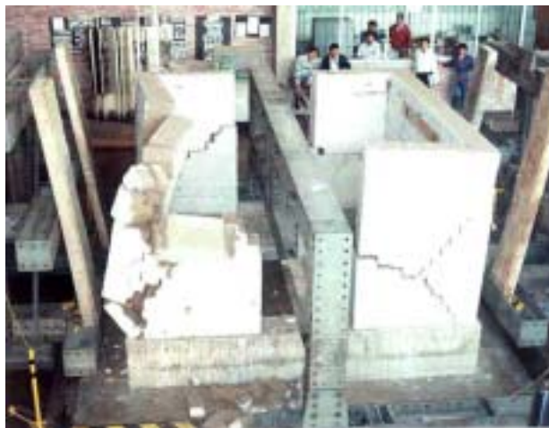
Figure 20 – Dynamic Testing of “U” Shaped Walls (Zegarra et al, 1997)
