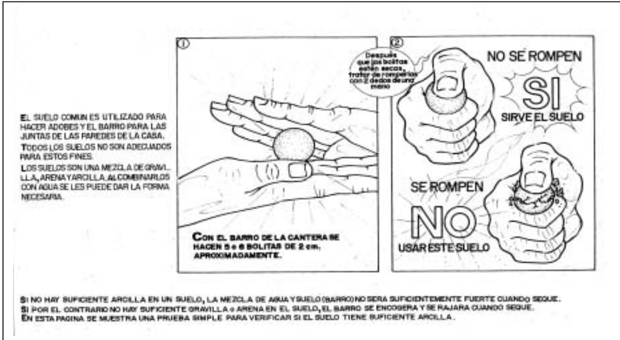
Figure 6 – Dry Strength Test (Pucp/Ciid, 1995)
