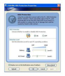
The protection level is temporally maximized 10 seconds after actions such as closing the LCD or unplugging the AC adaptor on the assumption that the notebook may be shortly picked up. The 3D sensitivity will also automatically go up as the tilt angle increases.
