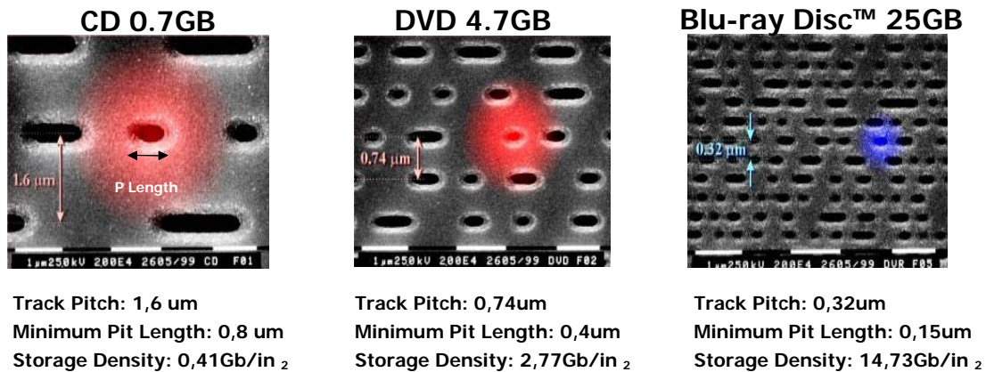
Fig.12-3 SEM photo of BD compared with CD and DVD
