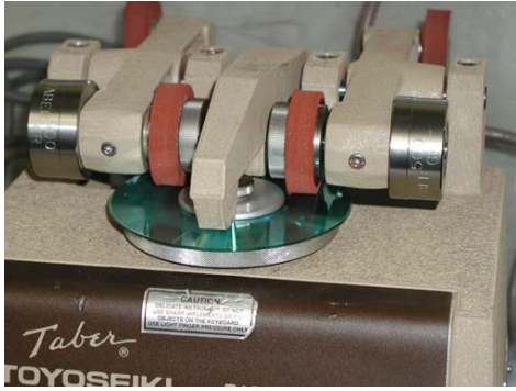
Fig.5-7 Taber abrasion test
