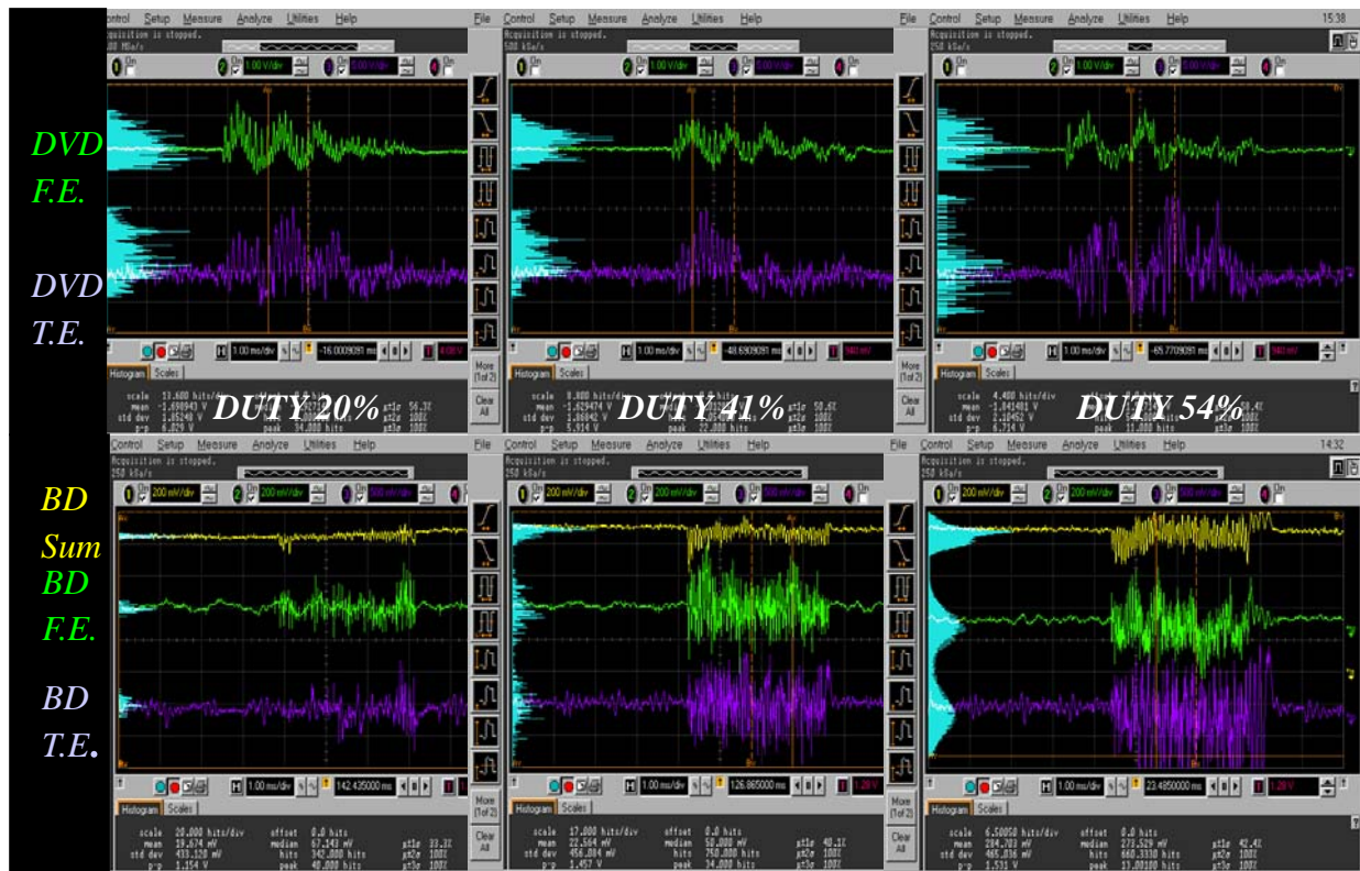
Fig.5-5 Example of the servo error signals of DVD player and BD player
