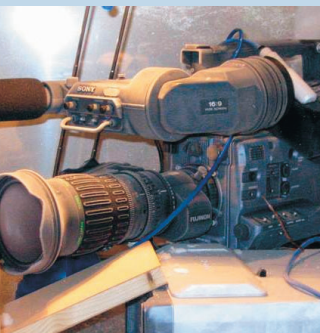
PDW-530 Camcorder record test at -22°F performed by WDR in Germany.
