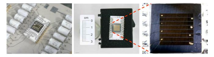
**Figure 3.** The 1 cm<sup>2</sup> CZT array sits on a dip package on a circuit board for a handheld gamma radiation spectrometer.
