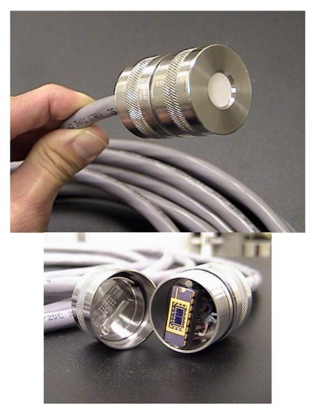
**Figure 5.** Stainless-steel waterproof package that houses the chemiresistor array. Left: GORE-TEX<sup>®</sup> membrane covers a small window over the chemiresistors. Right: Disassembled package exposing the 16-pin dual-in-line package and chemiresistor chip.
