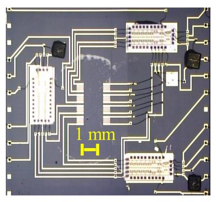
**Figure 4.** Four SAW sensor elements aligned vertically on an application specific integrated circuit. One delay line is left uncoated to compare frequency shifts of the other polymer or sol-gel coated lines.
