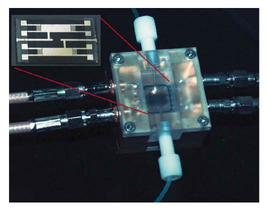
**Figure 7.** A miniaturized biosensor is shown consisting of a shear horizontal surface acoustic wave sensor coated with a molecular recognition layer. Highly specific coatings are used for biological warfare agent detection and medical diagnostics.
