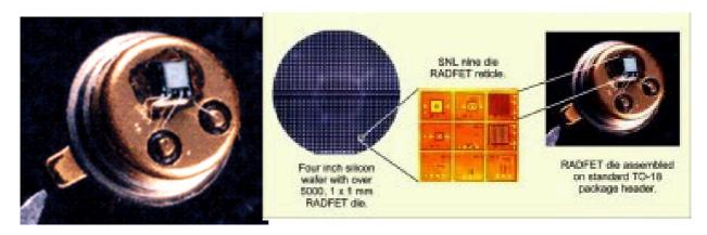
**Figure 2.** The 1 mm<sup>2</sup> RadFET element fits on a standard TO-18 package header. Over 5000 RadFETs can be microfabricated on a single 4 inch wafer.
