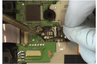
Figure 4.1: Example of installing a modification chip to bypass region locking (MaxConsole.net, 2007)
