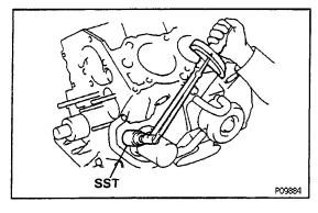
(b) Using SST, install the oil pressure sender gauge. SST 09818 - 30010
