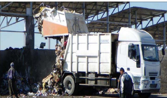
A garbage truck offloads trash at Solid Waste Transfer Station #1, located south of Kirkuk, Iraq. The $2.5 million facility has the capacity to handle 300 tons of waste per day. (USACE photo)
