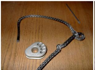
Next up, take the first inside out hole (the one closest to the tail's end) and un-invert it by pulling out the longer side of the rope (not the tail side of it)
