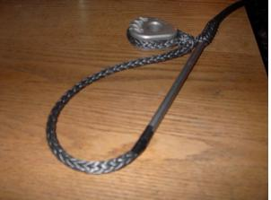
The next step is to « bury » the tail through the center of the line. You will need a splicing fid to do so. Start « burying » the line the closest you can from the noose of the splice and make sure you « bury » it far enough inside the line
