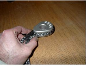
Now, wrap the rope around the thimble, starting from the inside out hole, to form your loop. It is important that you do not wrap the tail around the part but the other side of the rope; the longer side. Tighten it nicely and mark the other side of the rope where it meets with the inside out hole.
