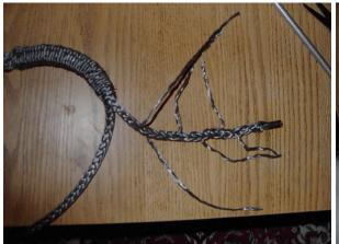
Here is the most important part of it, the tapering of the tail. Unbraid strands from the tail and cut them to varying length to form a perfect taper. For example, if you work with a 12 strand rope and your tail is 480mm long, divide 480 by 12 and cut a strand every 40mm.
