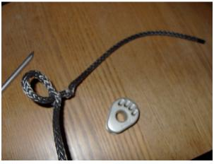
Exactly as you did on step 3, continue pulling on the tail until the rope is completly inside out.
