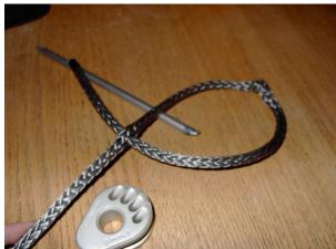
Feed the end of the tail through the new hole you just made.
