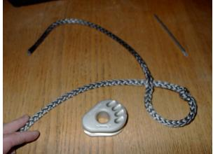
Continue pulling it out until the second inside out hole goes through the first one, as shown on the picture above.
