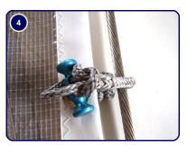
Pull the free spliced eye back over the EasyShackle<sup>™</sup> and tighten the Soft Hank in place
