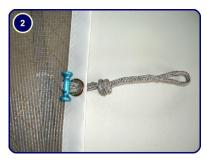
Lock the Soft Hank with a Double Overhand knot or a Figure-Eight knot
