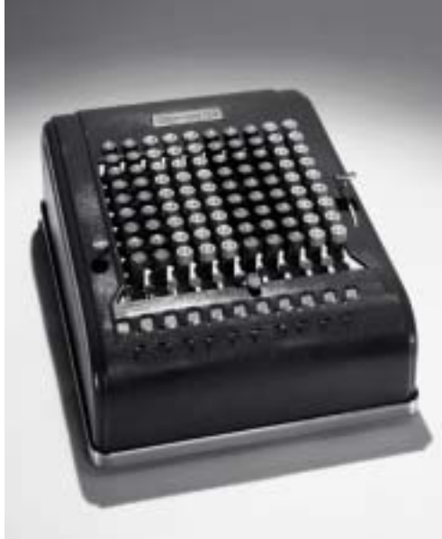
The comptometer, an early calculating machine, was an important piece of equipment at ADP in the pre-computer era.
