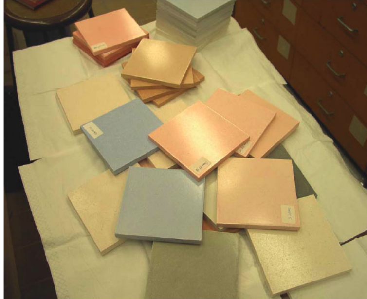
Decorative tiles made from sulfate-rich scrubber sludge and waste or broken tiles.
