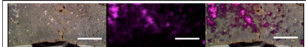
Figure 6.6. DUV excited H 2 O Raman map of an altered basalt from the Mojave desert, acquired from a 2 m standoff (image = 20.3 cm × 7.6 cm). Left: Visible reflectance image, white regions are composed of carbonates. Center: False-color map of the OH-stretch Raman band showing the distribution of hydrated minerals (magenta color) indicating extent of fluidic alteration. Right: Overlay of the reflectance and Raman map indicates carbonate deposited by aqueous transport and mixed with hydrous mineral phases. White scale bar: 5 cm.
