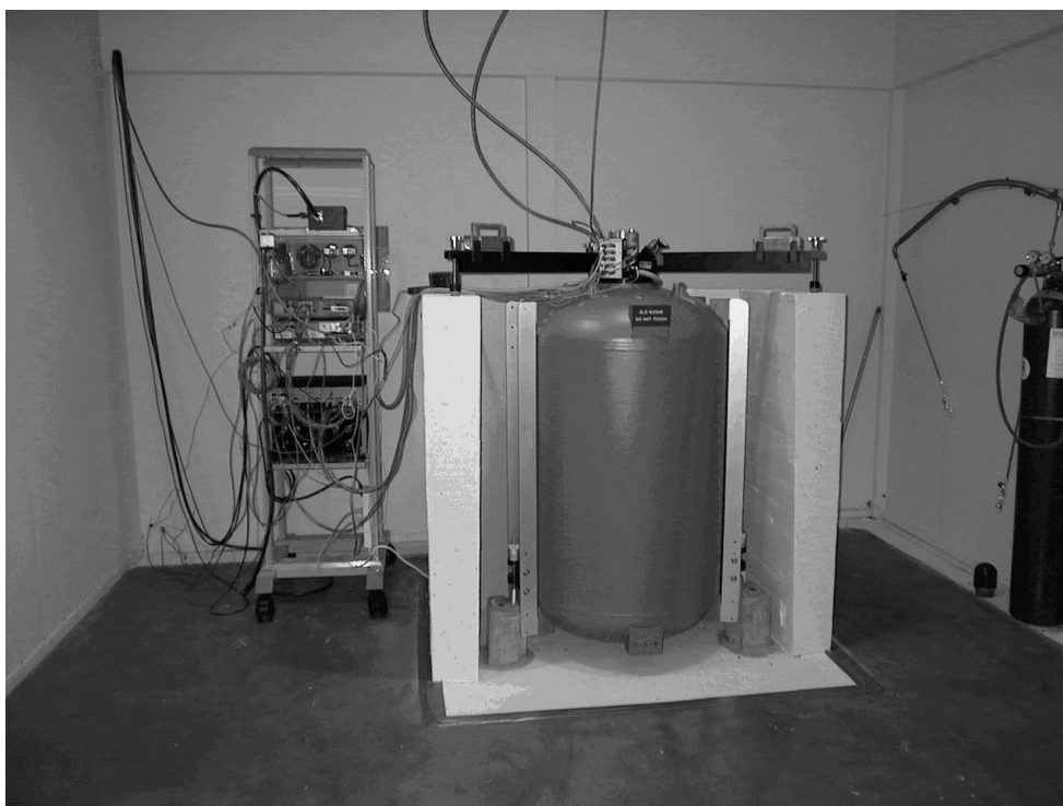
Fig. 1.1. Superconducting gravimeter T020 in gravity laboratory at Metsähovi.
