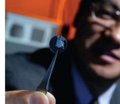
*Z.L. Wang, a researcher at Georgia Tech, is using nanowires to generate electricity. Such nanowire systems, assembled on surfaces as small as 2 square centimeters, could some day be used to power implantable medical devices.*
