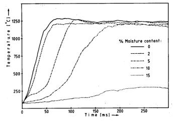
Figure 7. Temperature profiles of ternary mixtures with various moisture contents.
