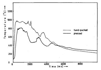
Figure 1. Temperature profiles of 12.5% charcoal/KNO<sub>3</sub> mixtures (pressed and hand-packed).
