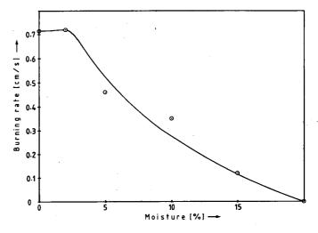
Figure 8. Burning rates of ternary mixtures with various moisture contents.
