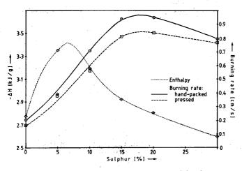
Figure 6. Enthalpy of reaction against percentage sulphur for ternary mixtures containing various proportions of sulphur.
