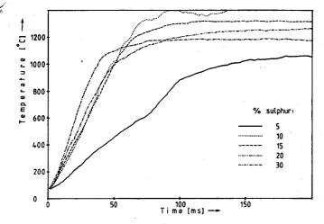
Figure 5. Temperature profiles of pressed ternary mixtures containing various proportions of sulphur.
