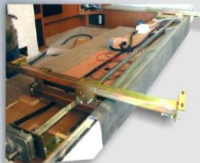
Dual Ram Rack and Pinion Slide Assembly in All Slide Outs
