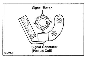
(e) Align the rotor tooth with the signal generator (pickup coil) projection.
