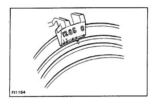
(c) Using a timing light, check the ignition timing. **Ignition timing:**
