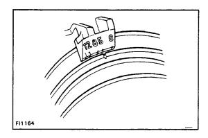
(b) Turn the crankshaft pulley until No. 1 cylinder is in compression stroke and the timing mark is aligned with 5 °6TDC mark.
