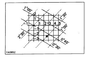
If camber and/or caster are not within specification, adjust by front and/or rear adjusting cams. (See Adjustment Chart)
